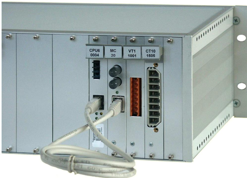
*Interconnection between the CPU module and the Media Converter module*
