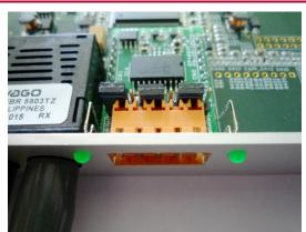
**JP1 is ON:** 120 Ω output impedance is *ON*
