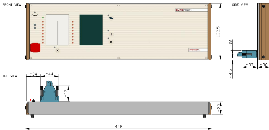
Figure 21-28 Dimensions for 84 HP wide remote HMI
