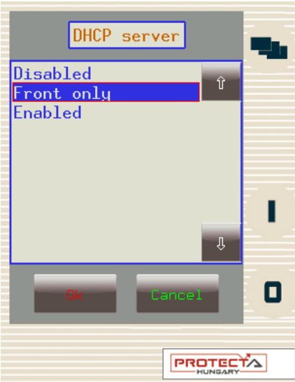
Figure 4-2 Enabling DHCP server for front panel control
