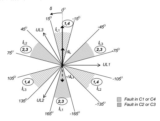
If the capacitor elements are not fused then the breakdown of a capacitor element will short-circuit a "layer" of capacitors. The capacitance increases and consequently also the capacitive current increases. This case was described in the explanation above.
