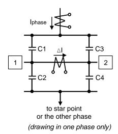
The capacitors in each phase are arranged in two branches with a current transformer connected between midpoints or close to midpoints of the two branches. Failures anywhere in the branches will cause an unbalance current to flow through the current transformer.
