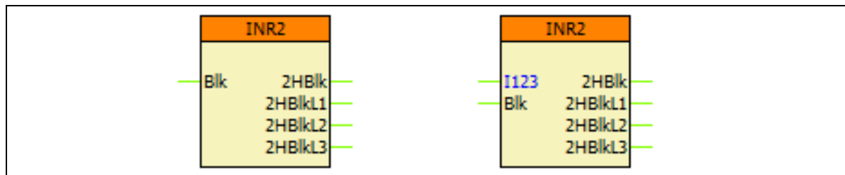
Figure 2-1 The function block of the inrush current detection function
