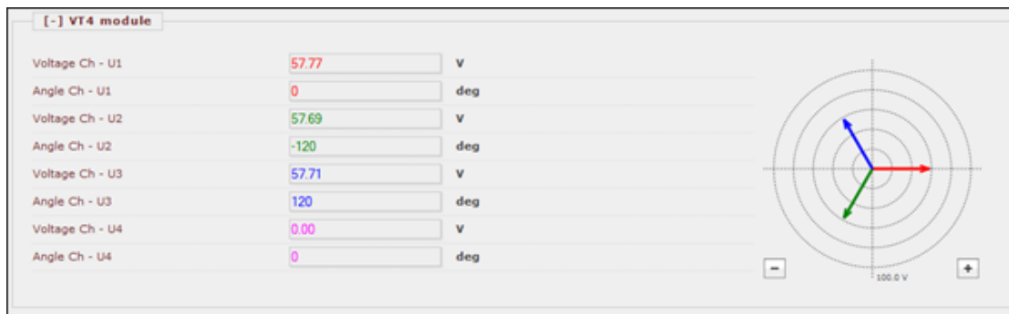
Figure 1-1 The measured secondary voltages and the vector diagram
