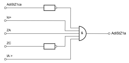
Fig. A-N fault detection
