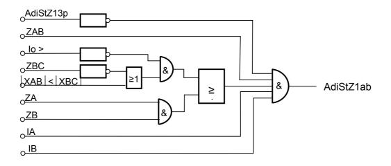
Fig AB fault detection
