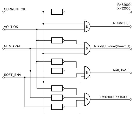
*Fig Z\_CALC internal logic*
