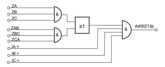
FigThree phase fault detection
