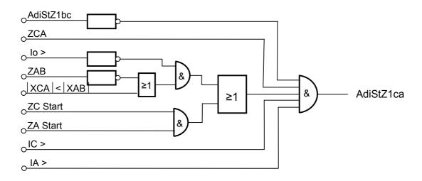
Fig. CA fault detection
