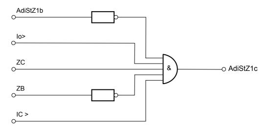
Fig. C-N fault detection
