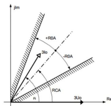
The output of the directional decision module is OK, namely it is TRUE if the phase angle between the residual voltage and the residual current is within the limit range defined by the preset parameter OR if non-directional operation is selected by the preset parameter (Direction=NonDir).
