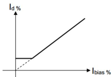
The horizontal axis of the operating characteristic is drawn as the percent of the phase current transformer rated current, the scaling of the vertical axis is in percent of the crated value of the current transformer into the differential branch.
