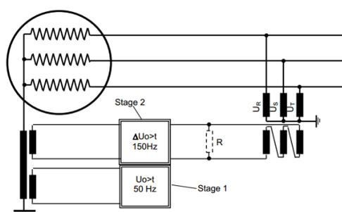
The EuroProt+ system applies a zero sequence overvoltage protection function (TOV59N) to perform the fundamental harmonic earth-fault protection. This function is described in a separate document.
