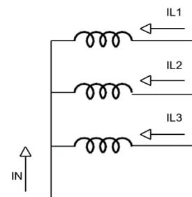
measured neutral current at the star point (IN) and the calculated zero sequence current component of the phase currents (IL1, IL2, IL3) and generates a trip command if the difference of these currents is above the characteristics.
