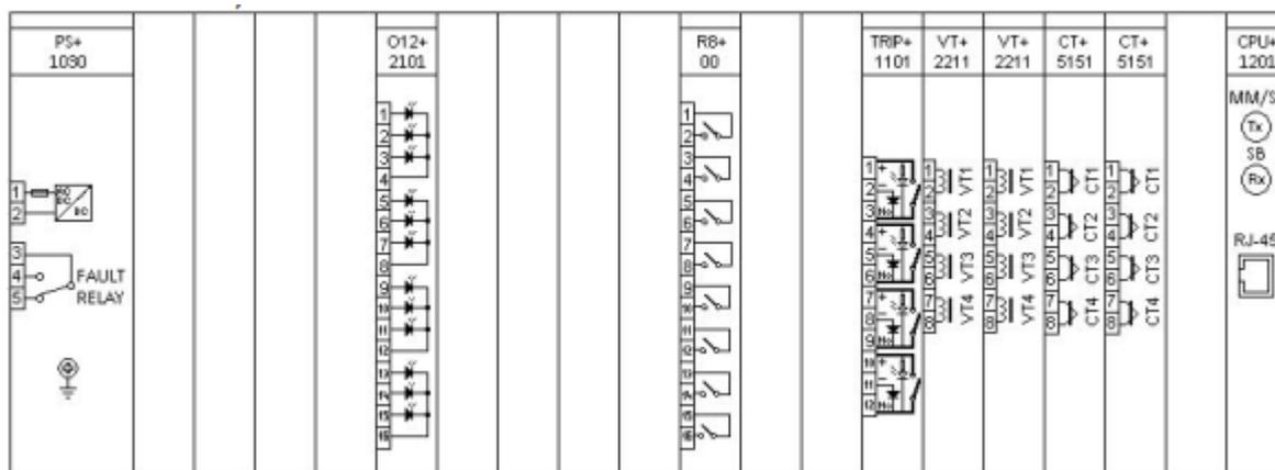
Basic module arrangement of the DTRV E9-Gen configuration (84TE, rear view)
