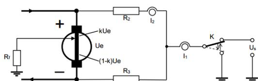
If only one of the poles of the excitation winding is available (e.g. in the case of excitation with rotating diodes) then the fault location and the exciting voltage cannot be calculated. The accuracy of the fault resistance calculation is however independent of these two factors. The applied algorithm is selected by parameter setting.
