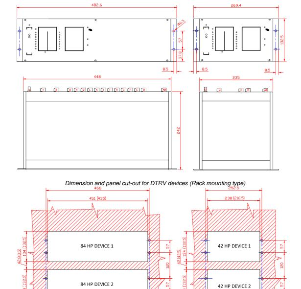
Note that rack mounting type devices can also be mounted in a cut-out (e.g. on a switchgear door). It is possible to mount them from the front or from the back of the cut-out. The dimensions for rack mounting cut-outs are in the figure below. Dimensions in brackets are applicable in case of mounting from the back.
