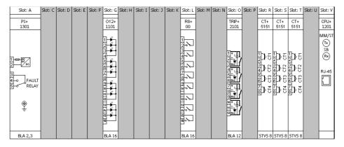
Basic module arrangement of the E4-TR configuration (84TE, rear view)
