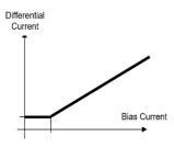
function. This curve is the function of the restraint (Bias) current, which is the maximum of the phase currents and the current of the neutral point.
