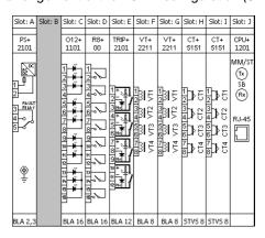
Basic module arrangement of the E3-TR configuration (42TE, rear view)
