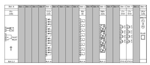
Basic module arrangement of the E1-TR configuration (84TE, rear view)
