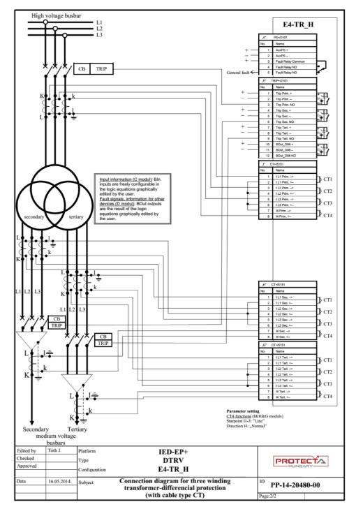
Typical connection diagram for E4-TR transformer differential protection
