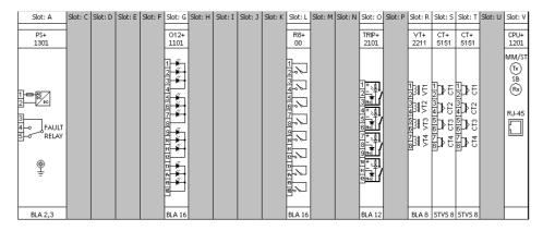
Basic module arrangement of the E2-TR configuration (84TE, rear view)
