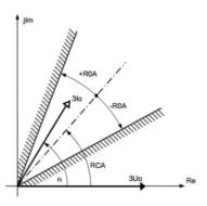
function block (51N/51Ns). This non-directional residual overcurrent protection function block is described in a separate document. The directional decision module calculates the phase angle between the residual voltage and the residual current. The reference signal is the residual voltage according to the Figure.
