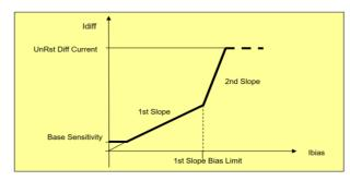
The characteristic curve has four sections. The first section is the base sensitivity, the second one serves to compensate the turns ratio deviation e.g. due to the operation of the on-load tap changer, the third is to eliminate false operation caused by the CT saturation and the fourth one is the unrestricted differential function.
