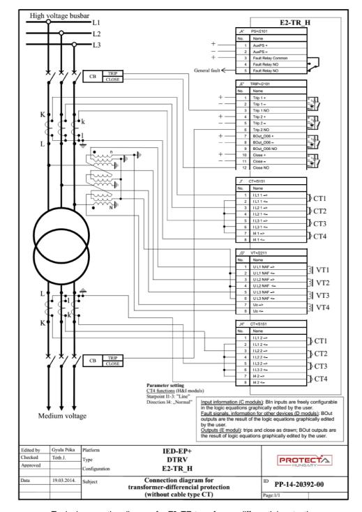
Typical connection diagram for E2-TR transformer differential protection
