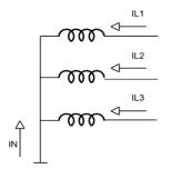
The function compares the measured neutral current at the star point (IN) and the calculated zero sequence current component of the phase currents (IL1, IL2, IL3) and generates a trip command if the difference of these currents is above the characteristics.
