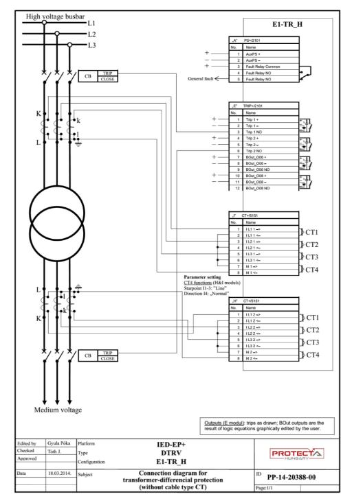
Typical connection diagram for E1-TR transformer differential protection
