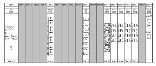
Basic module arrangement of the E3-TR configuration (84TE, rear view)
