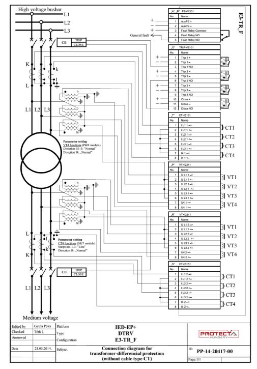
Typical connection diagram for E3-TR transformer differential protection
