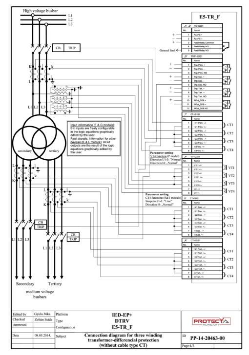
Typical connection diagram for E5-TR & E6-TR transformer differential protection
