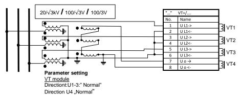
Figure 1-1 Example: Phase voltage and residual voltage measurement
