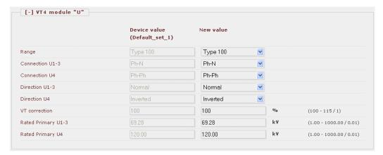
Figure 1-6 Example: Parameters for syncrocheck, using phase-to-pase voltage
