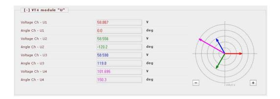
Figure 1-7 Example:On-line measurement for syncrocheck, using phase-to-phase voltage
