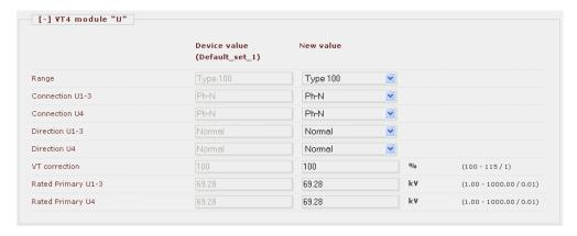
Figure 1-3 Example: Parameters for syncrocheck, using phase-to-neutral voltage
