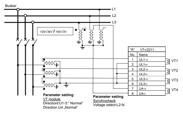
Figure 1-2 Example: Syncrocheck, using phase-to-neutral voltage
