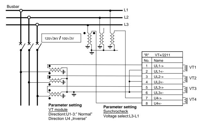
Figure 1-5 Example: Syncrocheck, using phase-to-phase voltage
