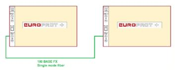
Transmission distance up to 2km if using multimode (shorthaul) fiber optic cable; and up to 120km if using single mode fiber optic cable (Long-haul, 1550nm)
