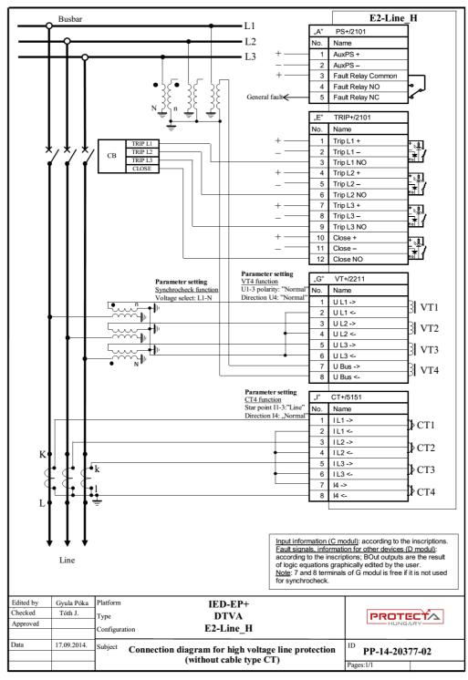
Typical connection diagram for E2-Line transmission line differential protection
