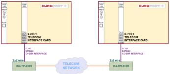
Communication via 2.048Mbit/s (E1/T1) Nx64kbit/s interface EuroProt+ devices support line differential communication via telecom networks with G703/704 2.048Mbit/s interface (E1). Besides, E1 in European networks the T1 interface (1.54Mbit/s) in America also available.
