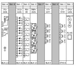
Basic module arrangement of the E2-Line configuration (42TE, rear view)
