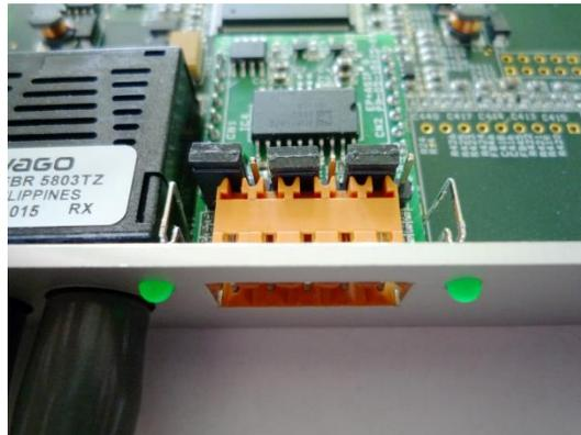
**JP1 is ON:** 120  $\Omega$  output impedance is *ON*
