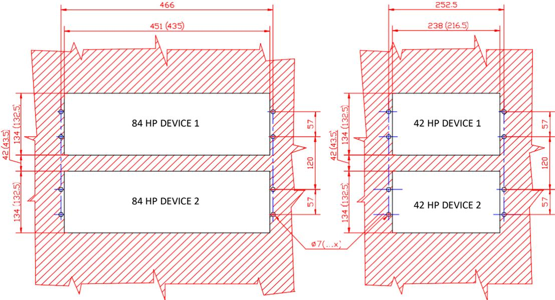
Note that rack mounting type devices can also be mounted in a cut-out (e.g. on a switchgear door). It is possible to mount them from the front or from the back of the cut-out. The dimensions for rack mounting cut-outs are in the figure below. Dimensions in brackets are applicable in case of mounting from the back.
