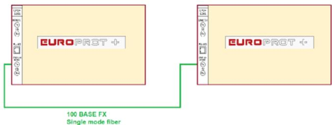
Transmission distance up to 2km if using multimode (short-haul) fiber optic cable; and up to 120km if using single mode fiber optic cable (Long-haul, 1550nm)
