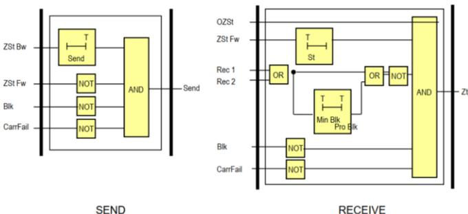
Direct underreaching transfer trip (DUTT)
