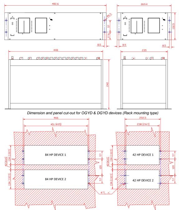
Note that rack mounting type devices can also be mounted in a cut-out (e.g. on a switchgear door). It is possible to mount them from the front or from the back of the cut-out. The dimensions for rack mounting cut-outs are in the figure below. Dimensions in brackets are applicable in case of mounting from the back.
