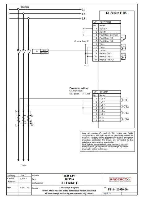
Typical connection diagram for the bay unit (distributed busbar differential protection)
