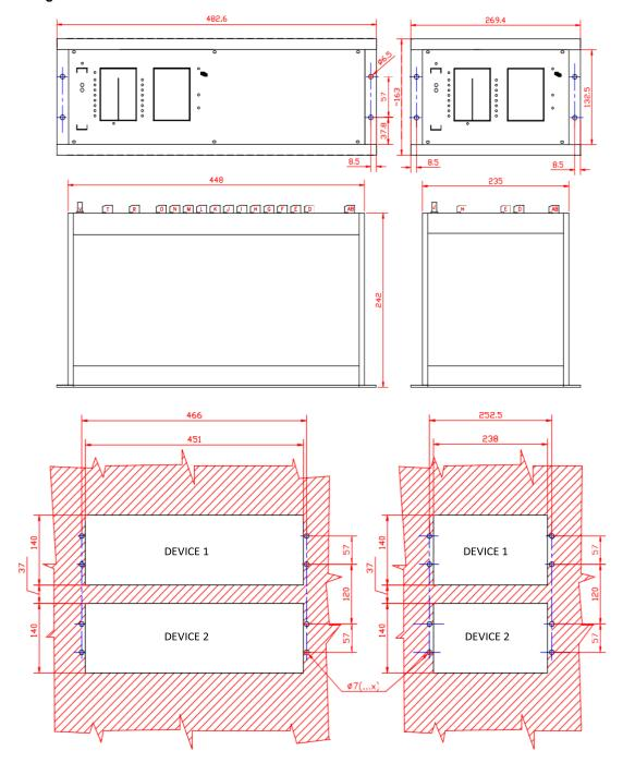
Dimension and panel cut-out for OGYD & DGYD devices (Flush mounting type)
