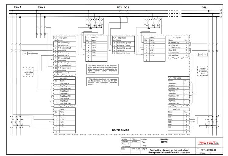
Typical connection diagram for the centralized three-phase busbar differential protection
