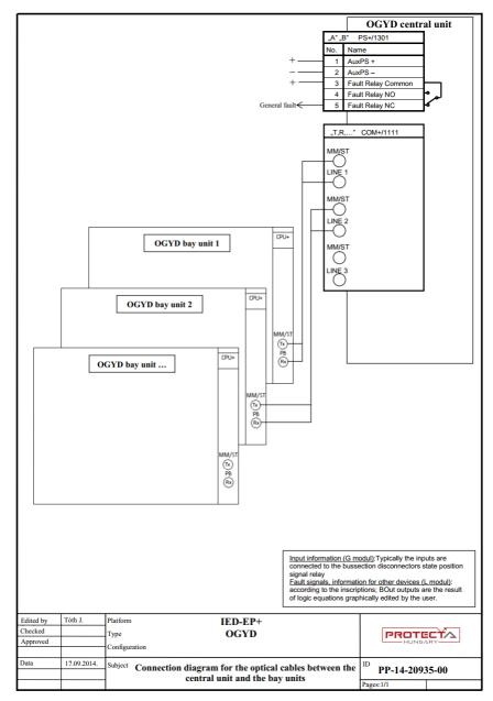
Typical connection diagram for the optical cable between the central unit and the bay units (distributed busbar differential protection)
