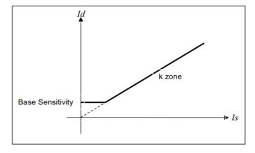
In case of detected through fault, the slope of the characteristic is dynamically changed to 90%. When tested, the applied method results a constant 90% measured value for the slope.
