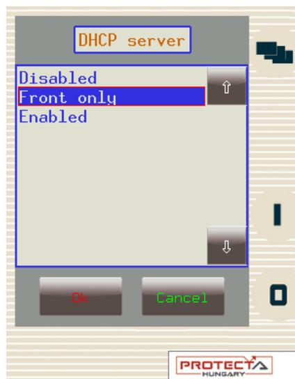
Figure 4-2 Enabling DHCP server for front panel control
