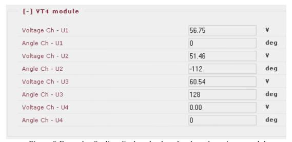
Figure 9 Example: On-line displayed values for the voltage input module
