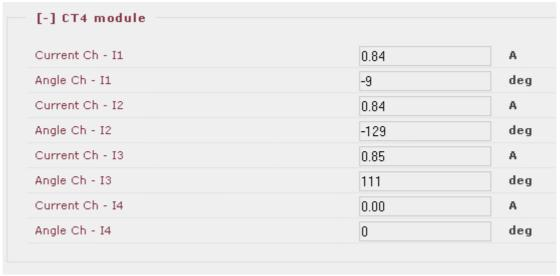
Figure 8 Example: On-line displayed values for the current input module
