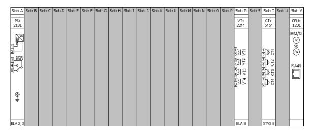
Figure 3 Basic module arrangement of the E2-BCU configuration (84TE, rear view)
