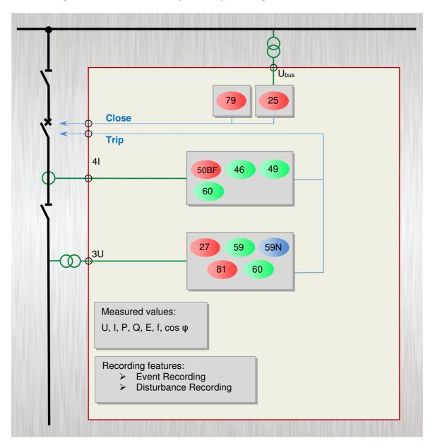
Figure 1 Implemented protection and control functions
