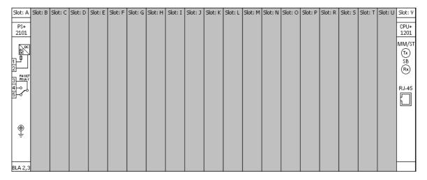
Figure 2 Basic module arrangement of the E1-BCU configuration (84TE, rear view)
