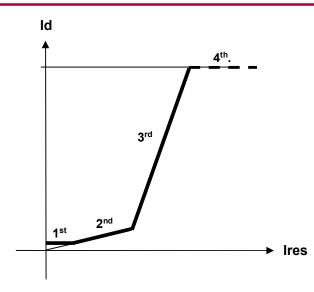
The characteristic curve has four sections. The first section is the base sensitivity, the second one serves to compensate the turns ratio deviation e.g. due to the operation of the on-load tap changer, the third is to eliminate false operation caused by the CT saturation and the fourth one is the unrestricted differential function. The slope of the third section is constant, it is 2.
