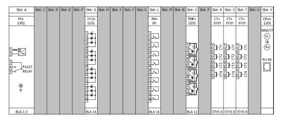
*Figure 1 Basic module arrangement of the E4-TR configuration (84TE, rear view)*
