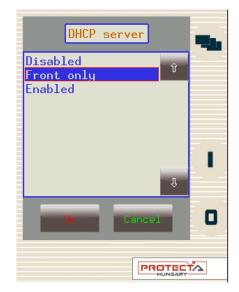
Figure 4-2 Enabling DHCP server for front panel control
