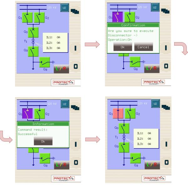
Figure 3-8 Closing Q1 disconnector
